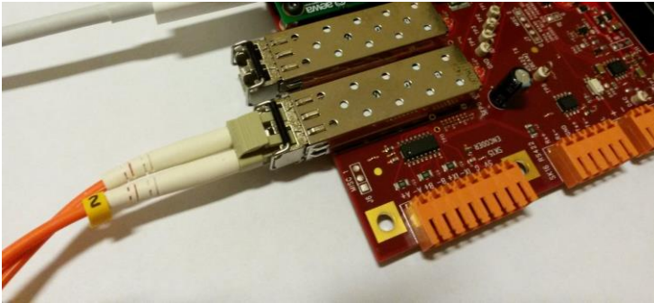
IMAGE 5 - OPTICAL FIBER CONNECTION WITH SFP MODULE
