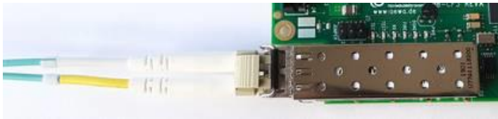
IMAGE 2 - OPTICAL FIBER CONNECTION WITH SFP MODULE
